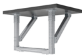
FASTENING OF THE FRAME WITH STRUTS TO THE REINFORCED CONCRETE SLAB
